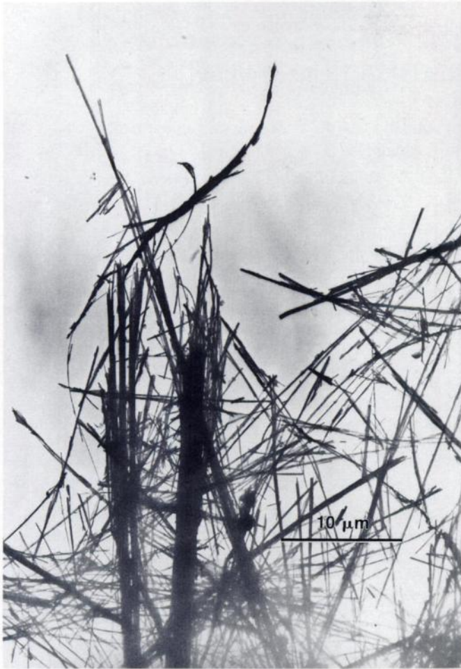
Fig. 4. Crocidolite asbestos in mainstream smoke from an original Kent cigarette. TEM; \times 3000 .
